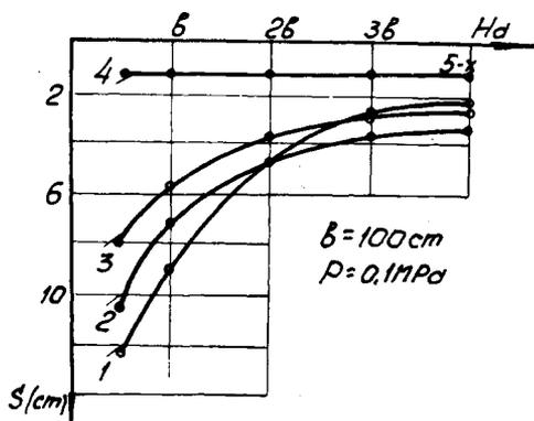
Fig.5. Plate settlements  $S$  versus thickness of the upper layer with different parameter  $n$ .
