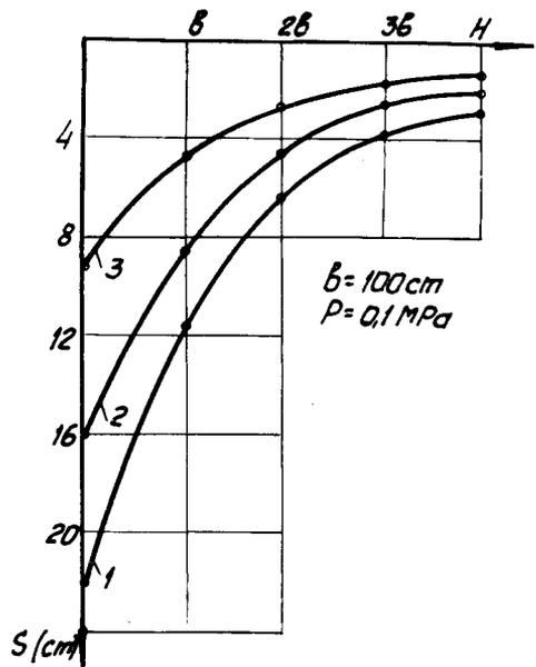
Fig.4. Plate settlements  $S$  versus thickness of the upper dense layer  $H_d$  with various thicknesses of the underlying layer  $H_w$ .
