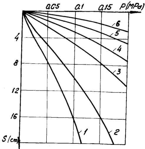
Fig. 2. Relations of the plate settlements (S) versus the load (P) for various thicknesses of the upper layer ( $H_d$ ) 1-thickness of the silty layer if b similar for other cases; 2-thickness of the upper layer  $0.5b$ ; 3-the same for  $2b$ ; 4-the same for  $3b$ ; 5-the same for  $4b$ ; 6-thickness of the sandy layer of  $5b$ .
