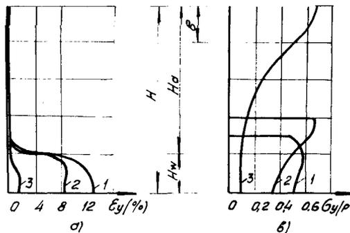
Fig. 3. Distribution of relative strains (a) and stresses (b) across the vase depth versus the upper layer thickness  $H_d$  with the similar thickness of the weak layer  $H_w=b$  and the load  $P=0.1$  MPa 1-thickness of the upper layer of  $0.5b$ ; 2-the same for  $b$ ; 3-the same for  $2b$ ; 4-the same for  $4b$ .
