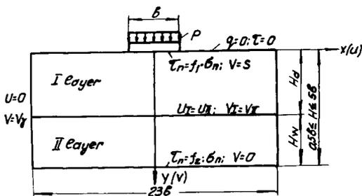
Fig. 1. Design scheme of the base
