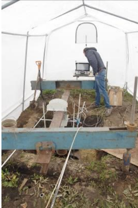
Fig. 9. 5000 cm 2 plate test: a – overview; б – test plate in the loading system: 1 – displacement sensor; 2 – load sensor; 3 – electro-mechanical drive.
