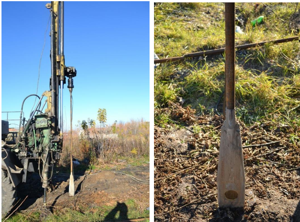
Fig. 16. Tests with a high-stiffness probe (RBT): a – general view; b – probe, equipped with one sensor
