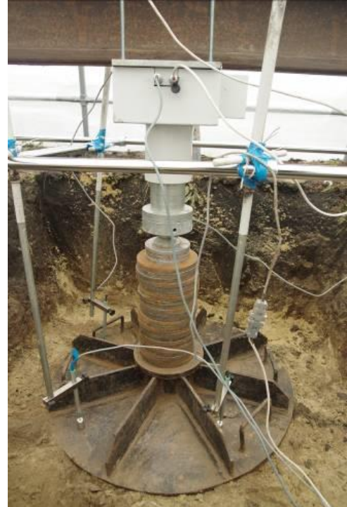
Fig. 9. 5000 cm 2 plate test: a – overview; б – test plate in the loading system: 1 – displacement sensor; 2 – load sensor; 3 – electro-mechanical drive.
