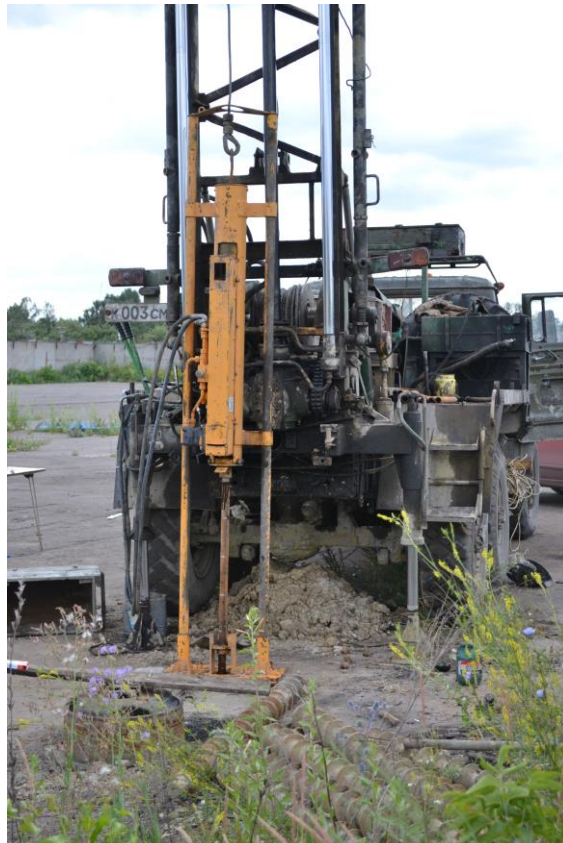
Fig. 8. Dynamic penetration tests with mounted “GEOMASH” equipment
