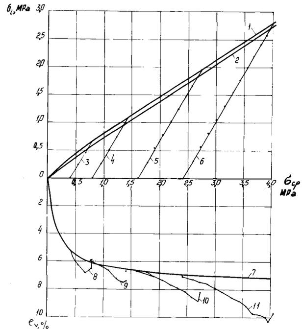
Fig.1. Loading trajectory curves and stress vs volume strain curves: Type I tests at  $I_D = 0$  ( $\gamma_s = 1.49 \text{ g/cm}^3$ )
