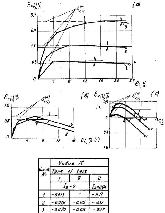
Fig.2 Dependence of the dilatant portion ( $\epsilon_v(i)$ ) of the volume strain on the shear strain intensity ( $\epsilon_i$ ): (a) Type I tests, (b) Type II tests at  $I_D=0$ ; (c) Type II tests, at  $I_D=0.94$
