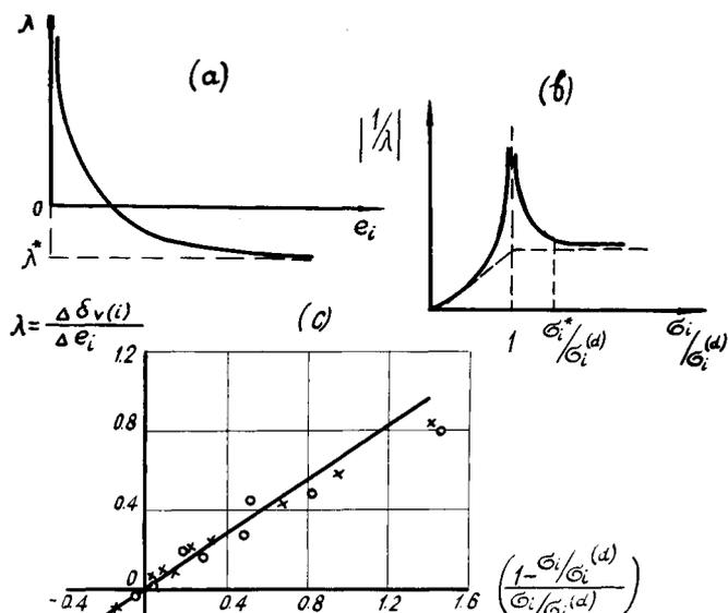
Fig. 3. Dependence of the rate of dilatancy ( $\lambda$ ) on the shear stress ( $\sigma_i$ ) and the shear strain ( $e_i$ ): (a)  $\lambda$  vs  $e_i$ ; (b)  $1/\lambda$  vs  $\sigma_i/G_i^{(d)}$ ; (c) Data of a Type I test at  $I_D=0$  ( $\gamma_s=1.49$  g/cm<sup>3</sup>);  $\circ$  -- at an initial hydrostatic pressure of 0.8 MPa;  $\bullet$  -- ditto, but at 1.6 MPa;  $\times$  -- ditto, but at 2.4 MPa
